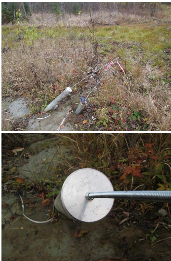
Figure 12-15: Miller Drillhole Collar & Cap for MI-19-35
