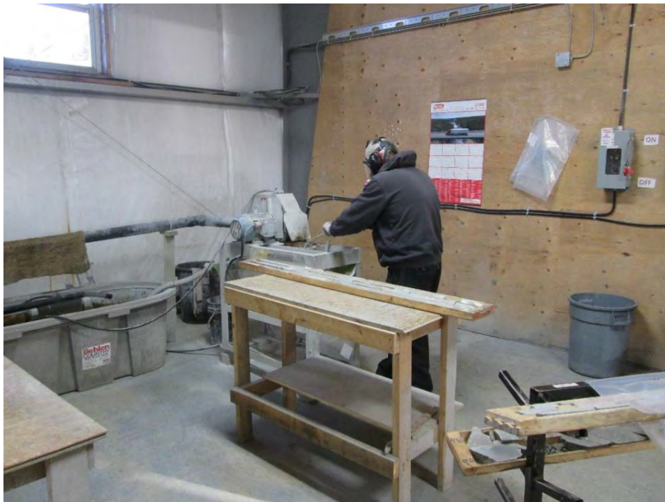
Figure 12-19: Drill Core Sample Saw
