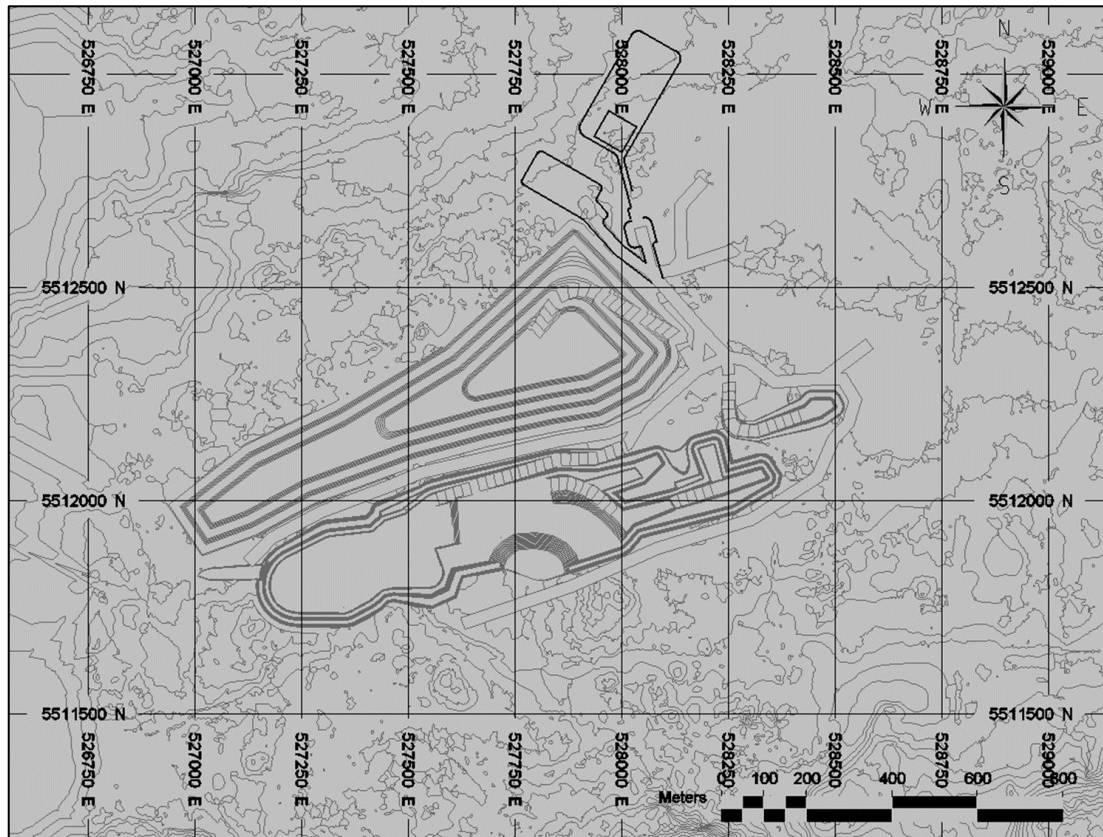
Figure 16-73: End of Year 13/14 Goliath Open Pit – Stockpile Removal Completed
