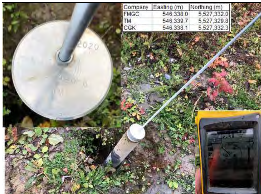
Figure 12-14: Drill Collar of Hole GL-20-016 showing the Capped Casing & Coordinates
