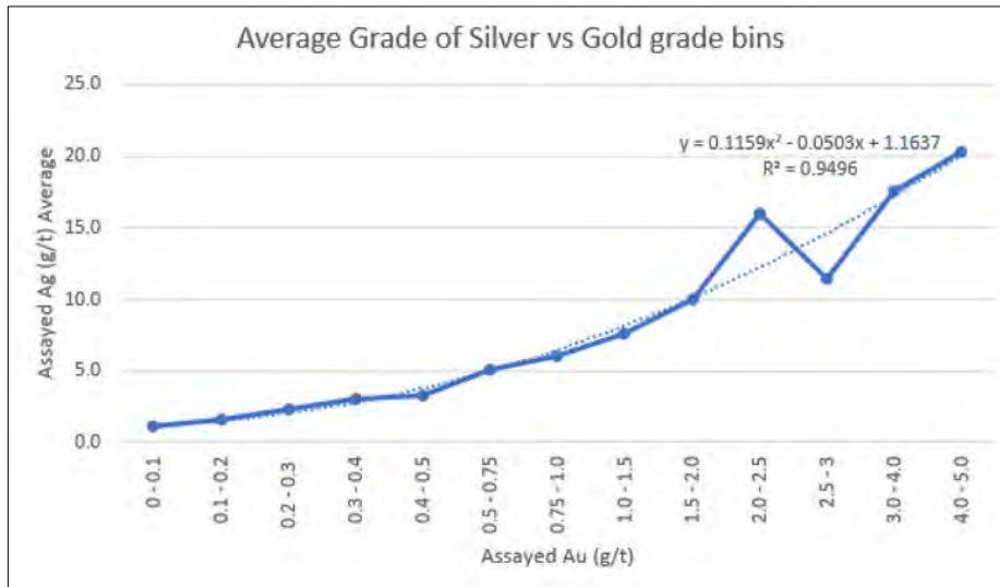
Figure 14-6: Formula to Calculate the Missing Silver Values
