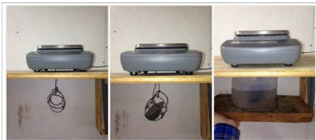
Figure 14-21: Specific Gravity Measurement Equipment Setup
