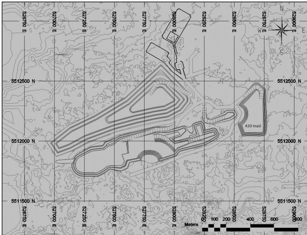
Figure 16-70: End of Year 11 – Goliath Open Pit – Stockpile Rehandle
